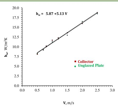
Figure 5: Deviation of h<sub>w</sub> of Collector from that of Unglazed Plate
