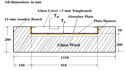
Figure 2: Indoor Experimental Single Glazed Collector
